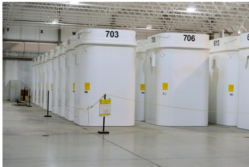
Figure 39: DSCs in Storage with IAEA Wire Seals
